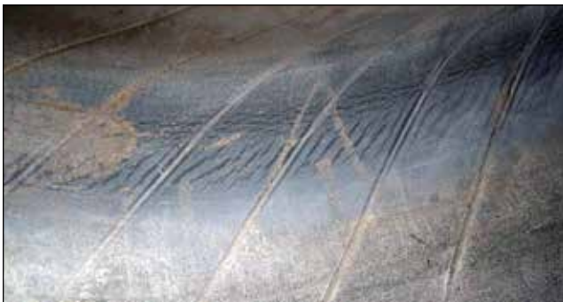
EFFECT: Inner Liner Marbling - Creasing CAUSE: Underinflation
