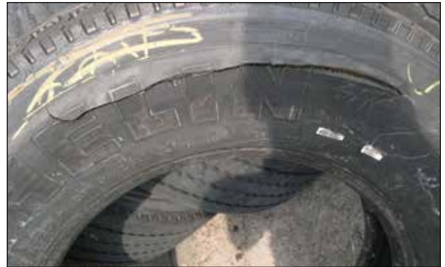
Fatigue Rupture or “Zipper”
